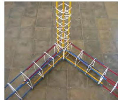
Figure 3. Bond Beam-Tie Column Connection Model. Note it has been suggested that to strengthen the interior corner, the interior long bars should pass through the joint and tie to the external long bars.
