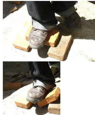
Figure 8. Three point bending test for brick strength, use average size Indonesian male, no bouncing
